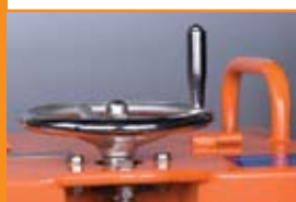
Hand wheel with endless screw depth control system
