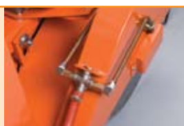
Water flow system on both sides of the blade
